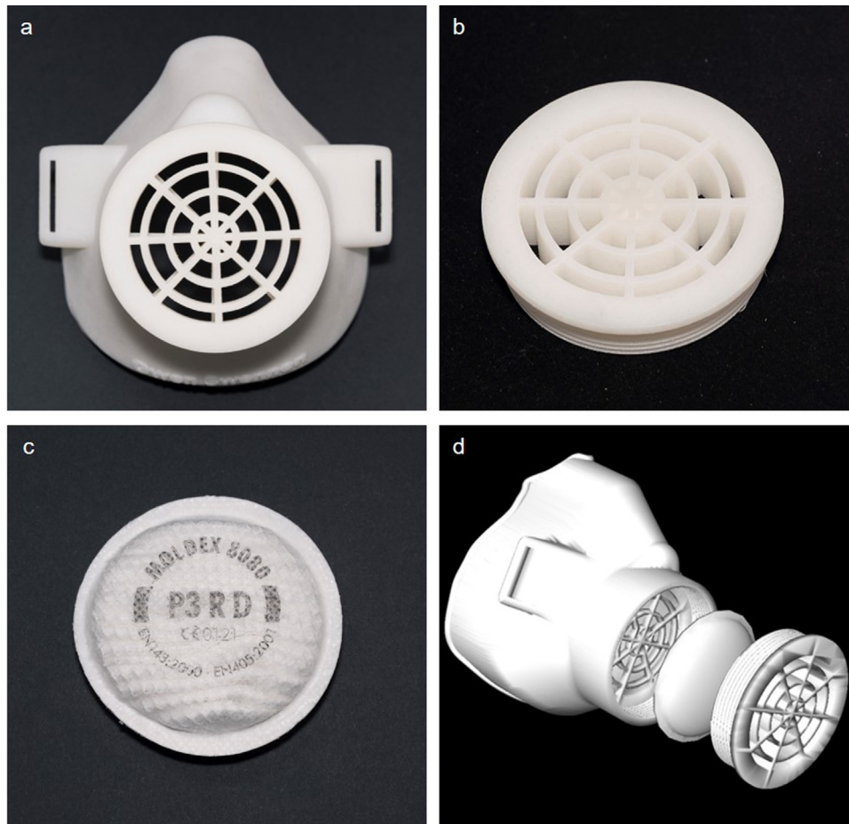
Fig. 1. Custom-made individualized 3D-printed protective face mask: (a) reusable 3D-printed face mask and (b) filter membrane support; (c) polypropylene (PP) non-woven melt-blown particle filter and (d) 3D image of the prototype.
